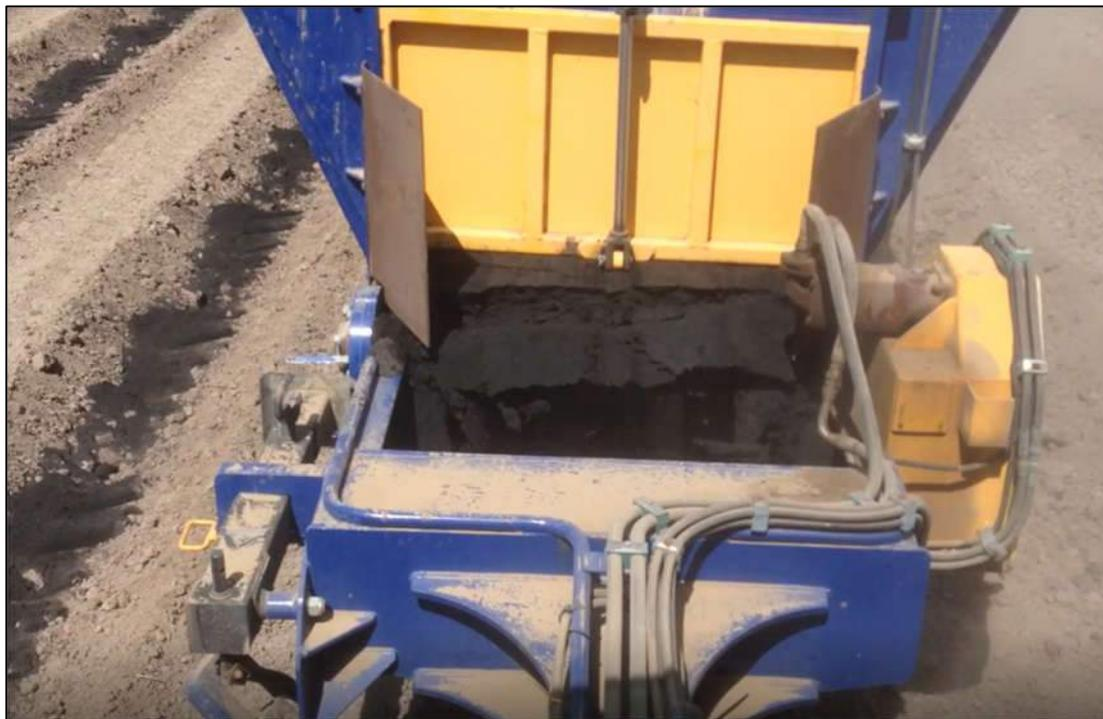
Figure 5 - Banded spreader used to apply mill mud
