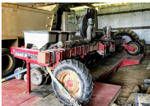
Fig.1 Soybean planter modified to place 3 rows on a bed
