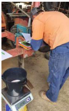
Anthony calibrating fertiliser box to correct rates
