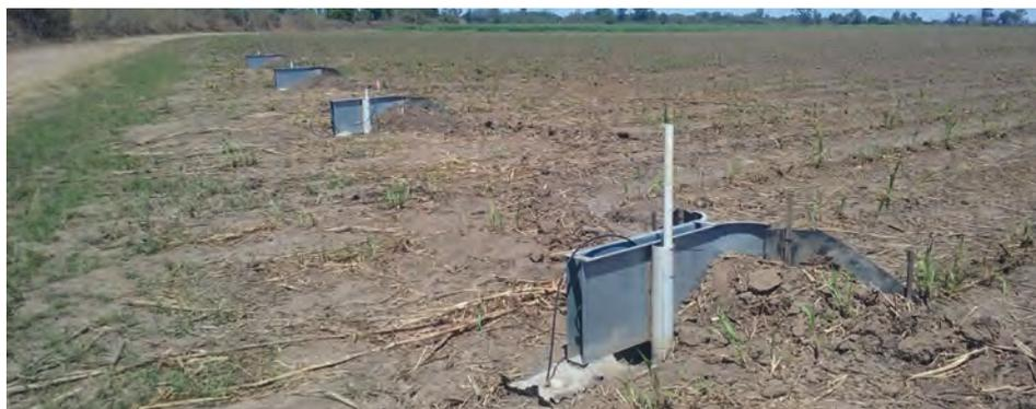
Above: Auto flumes at Ayr Farming Project Catalyst site measuring runoff flux (volume x concentration)
