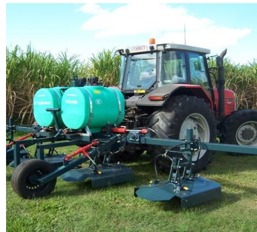
Lou's shielded sprayer set up for a 1.8m row controlled traffic farming system
