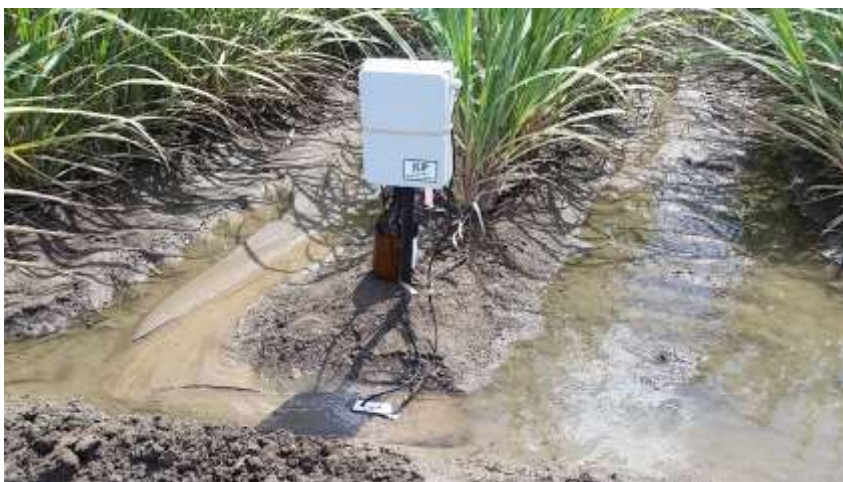
Photo 1: Kp sampler in action
