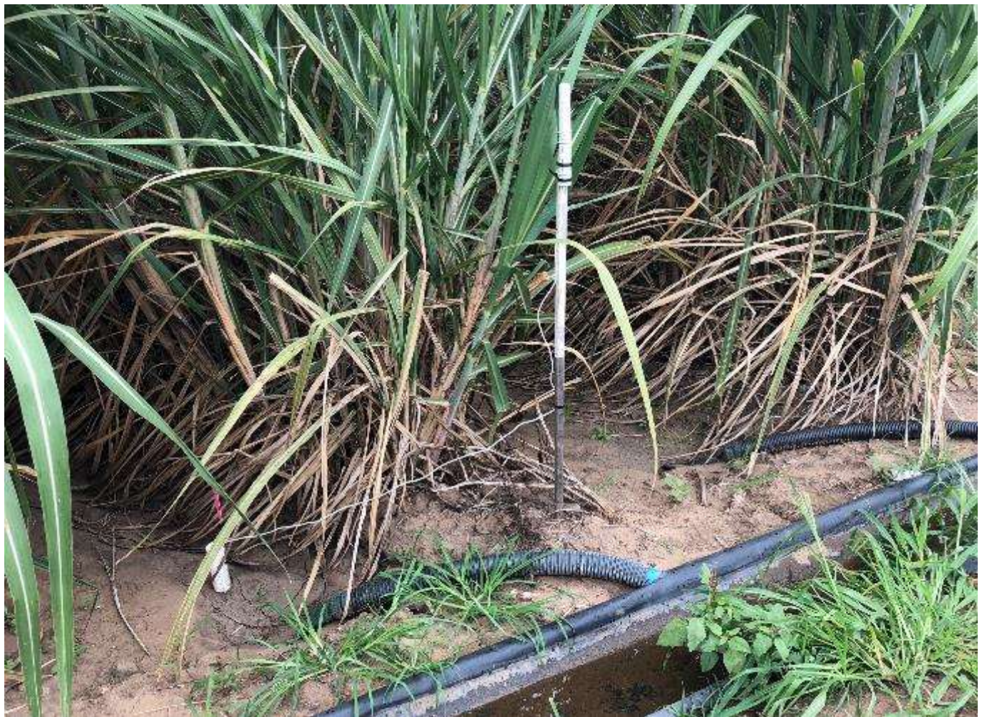
A sensor has been installed at the top of the block to record irrigations:
