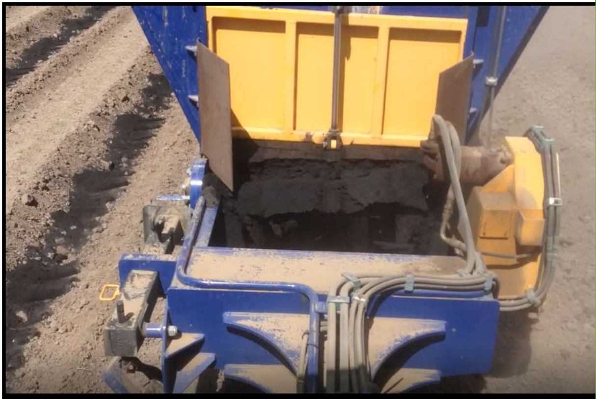
Figure 5 - banded spreader used to apply mill mud
